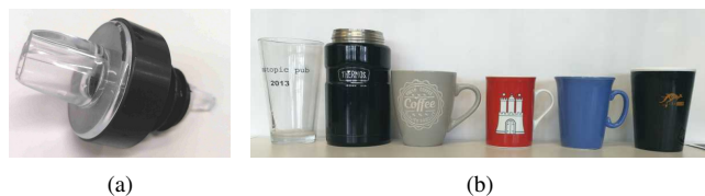
Fig. 4. (a) The spout equipped on the source container in robotic experiments. (b) From left to right, the first three target containers are the target containers in our datasets: a glass, a stainless steel cup, and a mug; the latter three target containers are the unseen containers used in robotic experiments: a red mug, a blue mug and a plastic cup.
