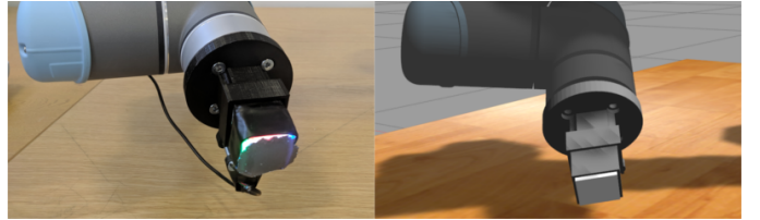
Fig. 1: Our experimental setup. Views of our real (left) and virtual (right) robot platform with a GelSight sensor mounted onto the end-effector of a UR5 robotic arm.
