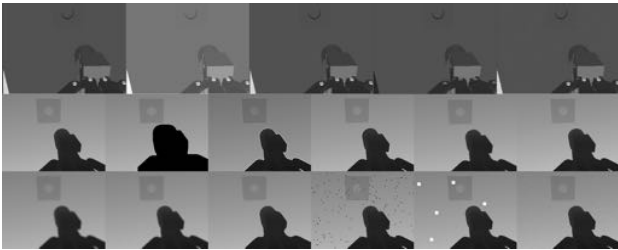
Fig. 4: Examples of used augmentations. Top row, left to right : original grayscale image, random brightness-contrast, motion blur, solarize filter, Gaussian noise. Middle row, left to right : original depth image, threshold and dilation, sharpening, embossing, motion blur, multiplicative noise. Bottom row, left to right : Gaussian blur, blur, median blur, coarse "pepper" dropout, coarse "salt" dropout, Gaussian noise.
